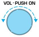
If the volume is set above a certain level and the ignition is turned off, the volume will come back on at a "nominal" listening level when the ignition switch is turned back on. If you wish to maintain your preset volume level, turn the audio system off with the power control before switching off the ignition.
